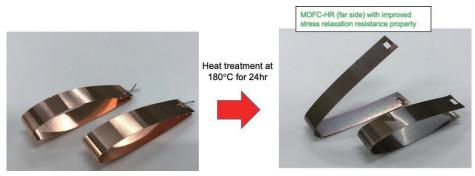
Heat resistance comparison between MOFC-HR (top strip) and conventional oxygen-free copper (bottom strip). MOFC-HR exhibits minimal degradation in properties even under severe thermal environments.
