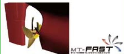
Attaching the MT-FAST pre-swirl stator improves a ship's fuel economy
