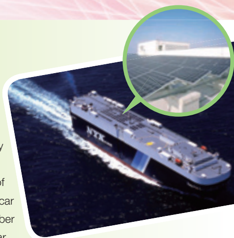
The car carrier equipped with the new solar power system
