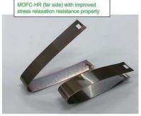
Heat resistance comparison between MOFC-HR (top strip) and conventional oxygen-free copper (bottom strip). MOFC-HR exhibits minimal degradation in properties even under severe thermal environments
